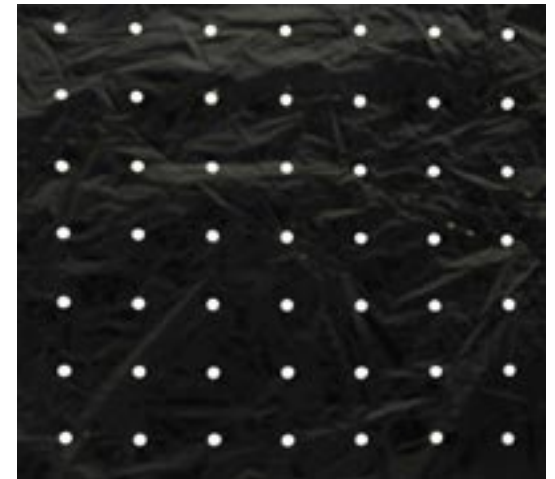
Photo of a section of a repetitive perforation pattern in aluminized mylar, typical of what can be done with the High-speed Pattern Cutter.
